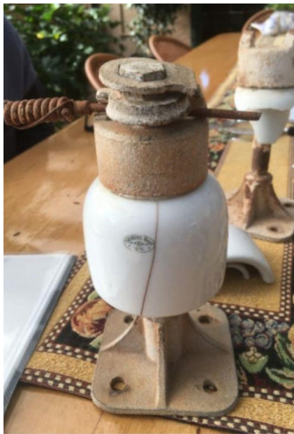
A surviving piece of the submarine cable at Port Augusta and one of Siemens' patented insulators: the flat spanner used to tighten the locking nut is still attached but the handle has broken off [Photos: Gavin Beinke]
