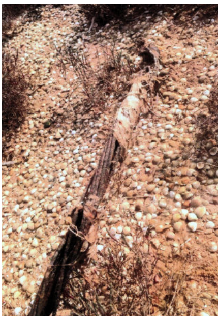
A surviving piece of the submarine cable at Port Augusta and one of Siemens' patented insulators: the flat spanner used to tighten the locking nut is still attached but the handle has broken off [Photos: Gavin Beinke]
