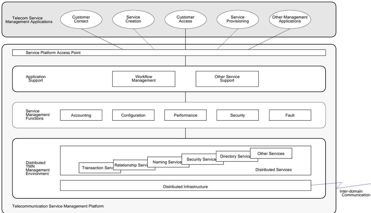
Figure 6: Telecommunication Service Management Platform
