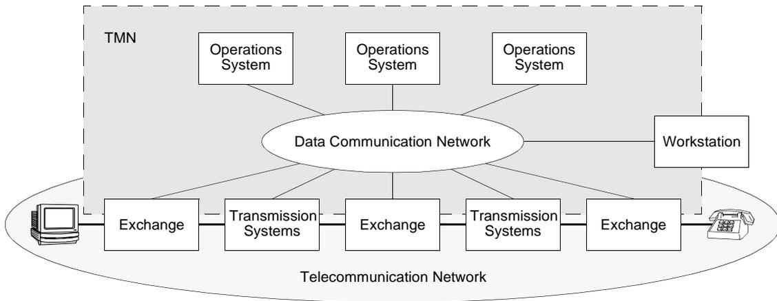
Figure 1: Relationship of TMN and Telecommunication Network
